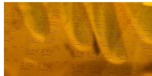
Figure 5. a) SiC wafer that has been stripped of seed layer and nickel mask. Note the wafer is transparent once again. b) Cavities of the wafer can be seen up close from the etching process.
