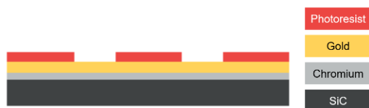
Figure 2. Not-to-scale representation of SiC wafer after pattern is developed.
